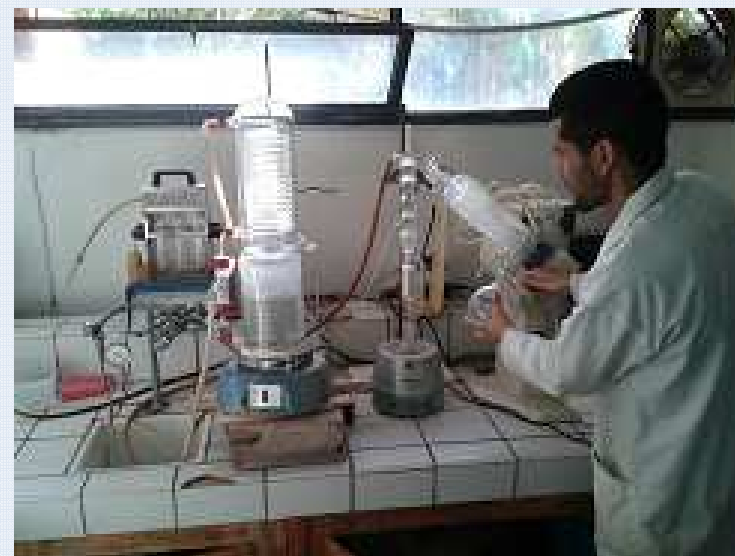
Oil extraction using the Soxhlet method
